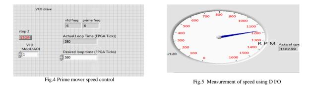
Speed of the prime mover is sensed by a encoder mounted on the shaft of DFIG system. Quadrate encoder outputs are being given to NI 9403 card and the digital output of encoder being converted into corresponding speed. Speed of the prime mover is sensed and displayed on the front panel as shown in Fig 5.
