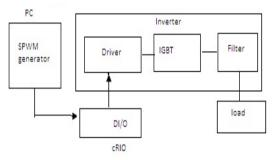
Fig.2 Block diagram for driving signals generation from cRIO
