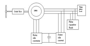
Fig.1 Wind Energy conversion system based on DFIG
