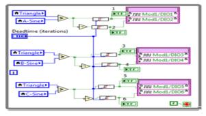
Fig.3 LabVIEW VI for sine PWM
